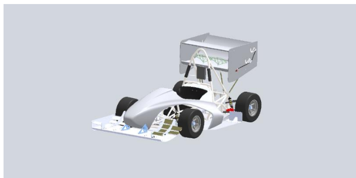
Rys.1. Model bolidu wraz z pakietem aerodynamicznym klasy Formula Student Fig.1. Model of a Formula Student car with aerodynamic package
