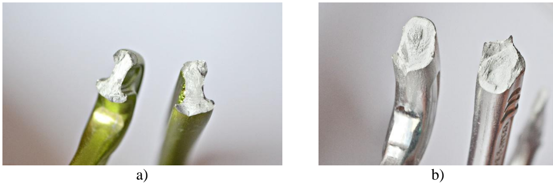
Rys. 3. Złom: a) ClimbX Ultra Wire Straight Gate, b) Camp HMS Lock Fig. 3. Fracture surface: a) ClimbX Ultra Wire Straight Gate, b) Camp HMS Lock
