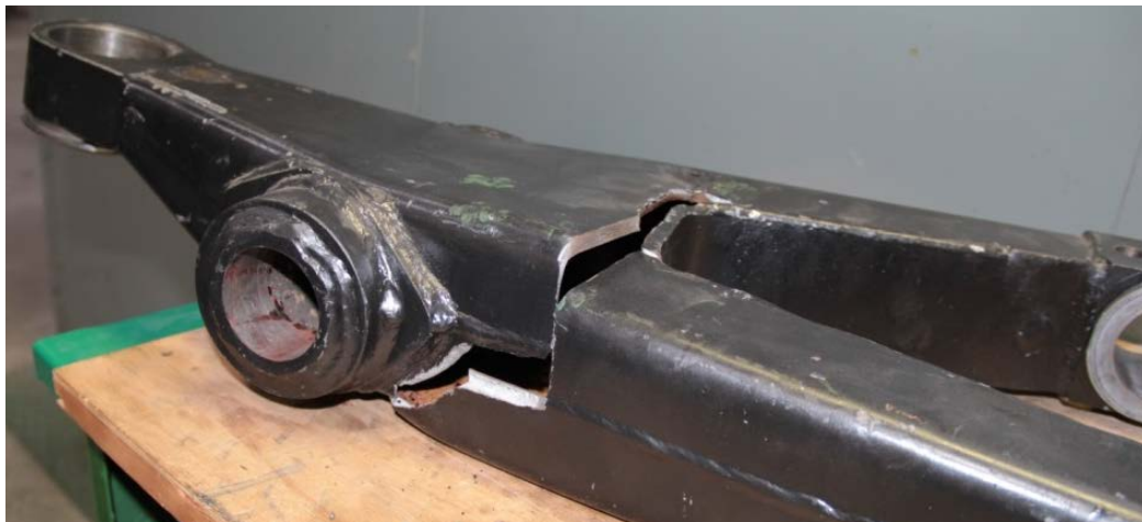
Fig. 1. The nature of the lower suspension arm failure
