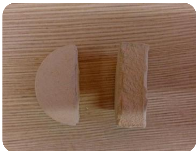
Fig 1. Porous ceramic skeleton made on the basis of fly ash
