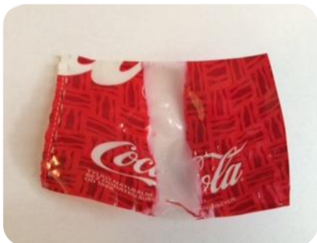
Fig. 1. A fragment of the waste packaging film from the Coca-Cola drink, with the visible area of the varnish coating removal
