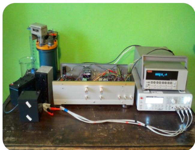
Fig. 1 Test stand for impedance measurements of electrochemical cells
