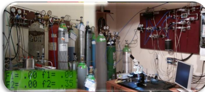
Fig. 1. A system for dosing gas mixtures for testing chemical gas sensors
