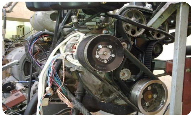
Fig. 1. Electric machine supporting the combustion engine installed on the laboratory stand.
