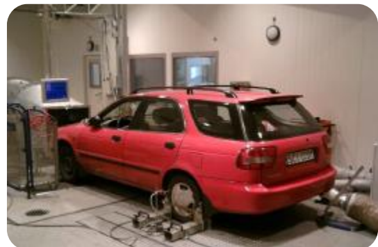
Fig. 2. Testing of Smart Hybrid system components on a chassis dynamometer.
