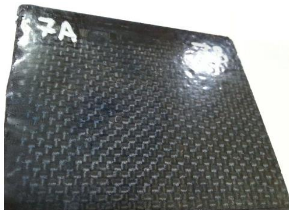
Fig. 2. Composite for protection against electromagnetic radiation.
