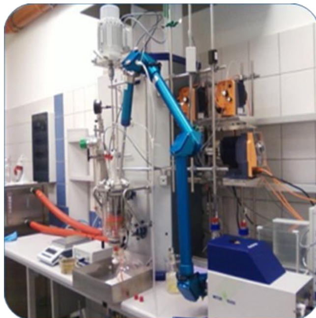
Fig 1. Automatic reactor with FTIR analytic module.
