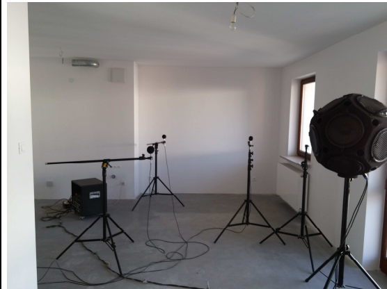
Fot. 2. Field measurements of airborne sound insulation between rooms.
