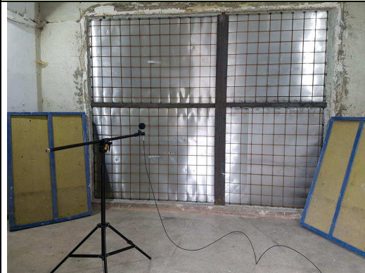
Fot. 1. Laboratory measurement of sound insulation of building elements. Measurement of airborne sound insulation.
