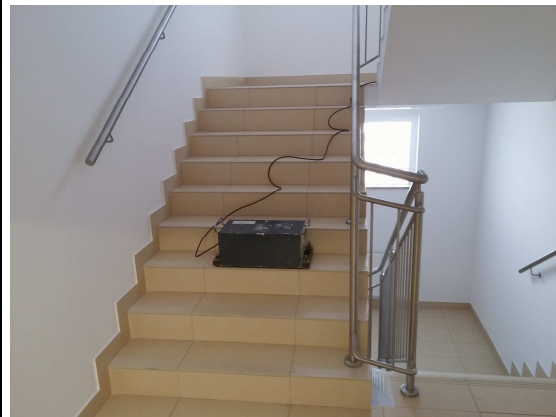
Fot. 3. Field measurements of impact sound insulation.
