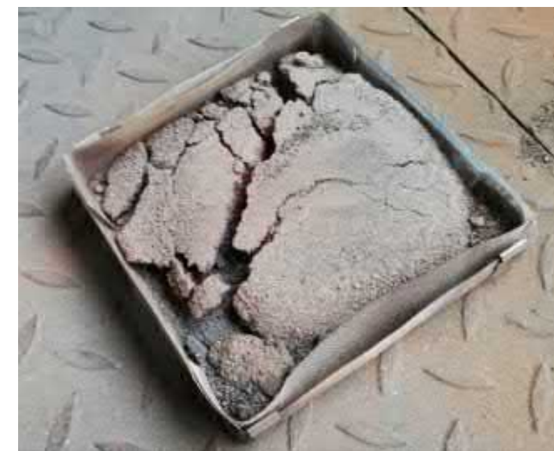
Samples of fly ash before and after ammonia desorption tests
