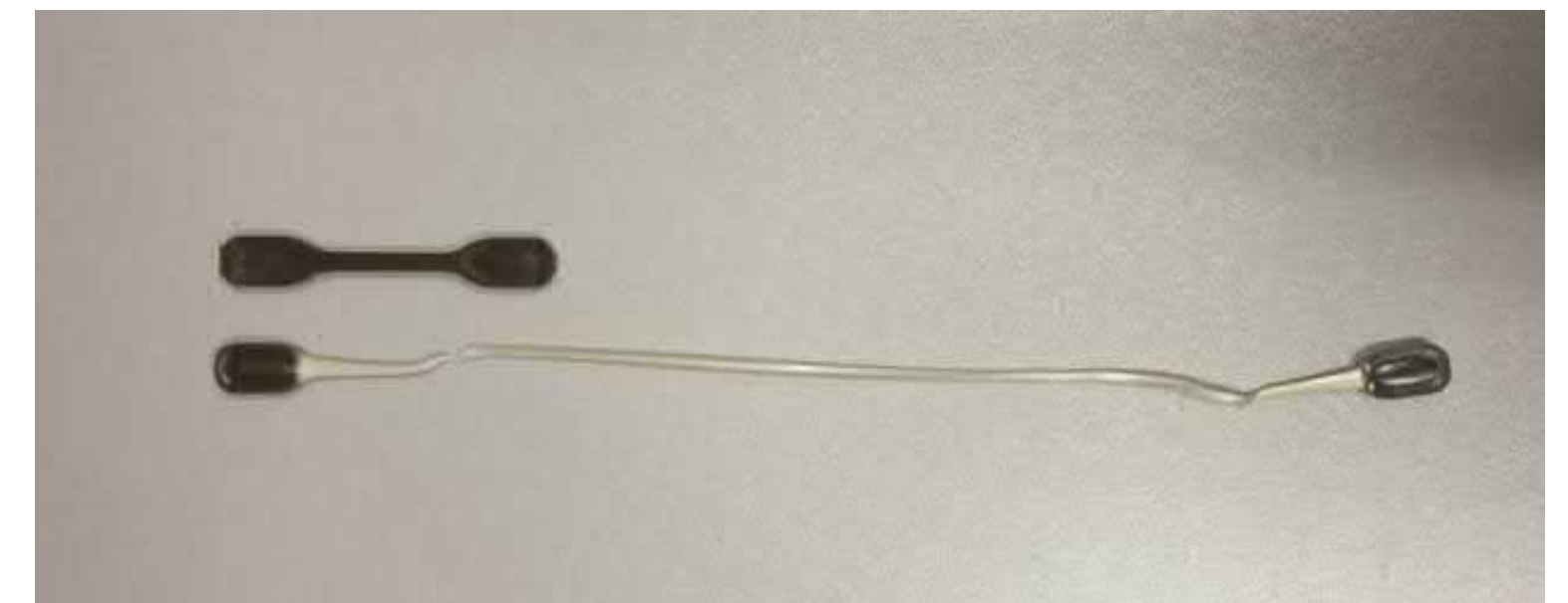
The LLDPE samples with the addition of 5% ash, before and after testing on a testing machine
