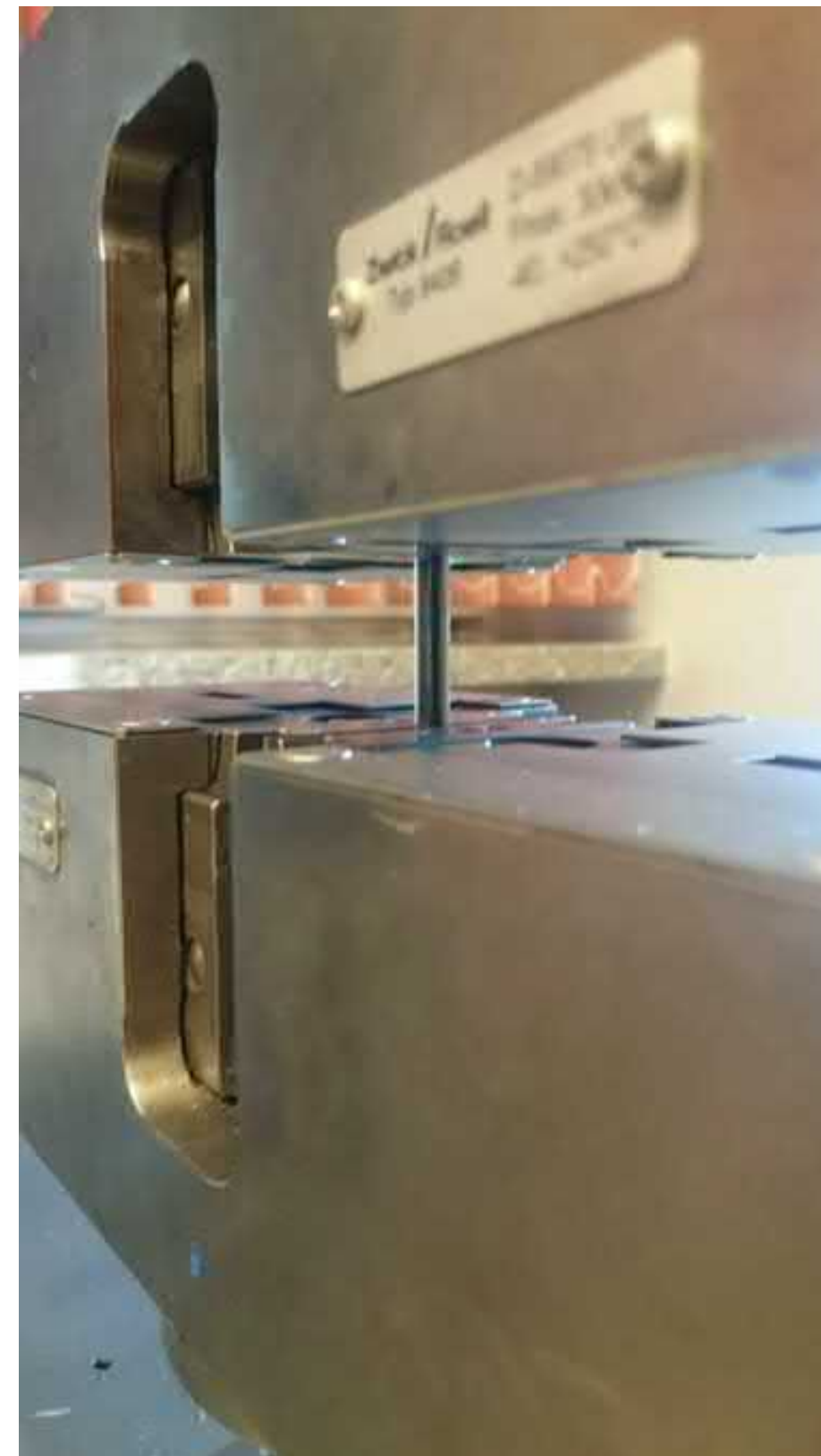
The course of the test on the testing machine - tested LLDPE sample with the addition of 5% ash.
